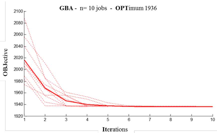
Fig. 6 The performance of the GBA for n=10 and h=0.2 - optimum value 1936 (tuning under parameters: ns=50 ; nb=5 ; ne=3 ; nrb=5 ; nre=5 ; ngh=5 ).
