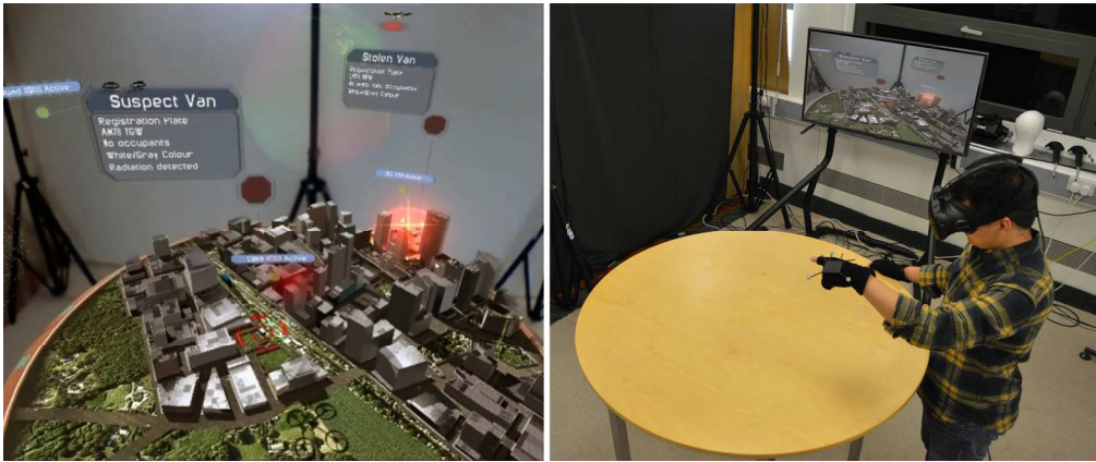
Figure 2: Mixed Reality Command and Control Concept Demonstrator – the MxR user (right image) is able to see the 3D cityscape scenario (left image) via the HMD and can interact with the displayed features and information panels using gestural commands, including sweeping motions on and around the otherwise empty table shown.
