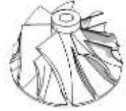
Figure 8: Turbine wheel (image source: Baumers)
