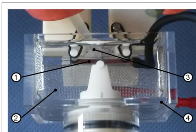
**FIGURE 1 |** Set-up of the electrochemical cell for corrosion fatigue experiments, including the sample (1) as working electrode, a fine platinum mesh (2) as counter electrode, an agar salt bridge (3) connected to the saturated calomel electrode reference electrode and an acrylic glass container (4) filled with 0.01 M Na<sub>2</sub>SO<sub>4</sub> + 0.01 M NaCl.
