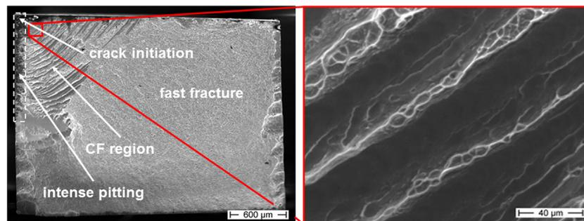
**FIGURE 7 |** Fracture surface of a corrosion fatigue (CF) sample tested at an anodic potential of  $0$  mV,  $\sigma_a = 388$  MPa, and  $N_f = 2,616$ , in  $0.01$  M  $\text{Na}_2\text{SO}_4 + 0.01$  M NaCl (tensile loaded surface is at the top, detailed view of striated corrosion fatigue region showed in red inset).
