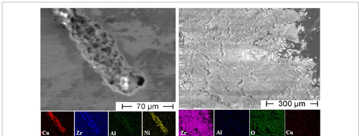
**FIGURE 8 |** Energy dispersive X-ray analysis of a corrosion pit at the side surface of the bending sample (left) and of the dissolved material extracted from the electrolyte as powder after testing (right).
