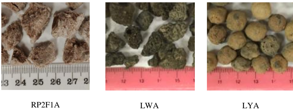
143 Figure 1: Various types of coarse aggregate used in this study (RP2F1A, LWA and LYA)
