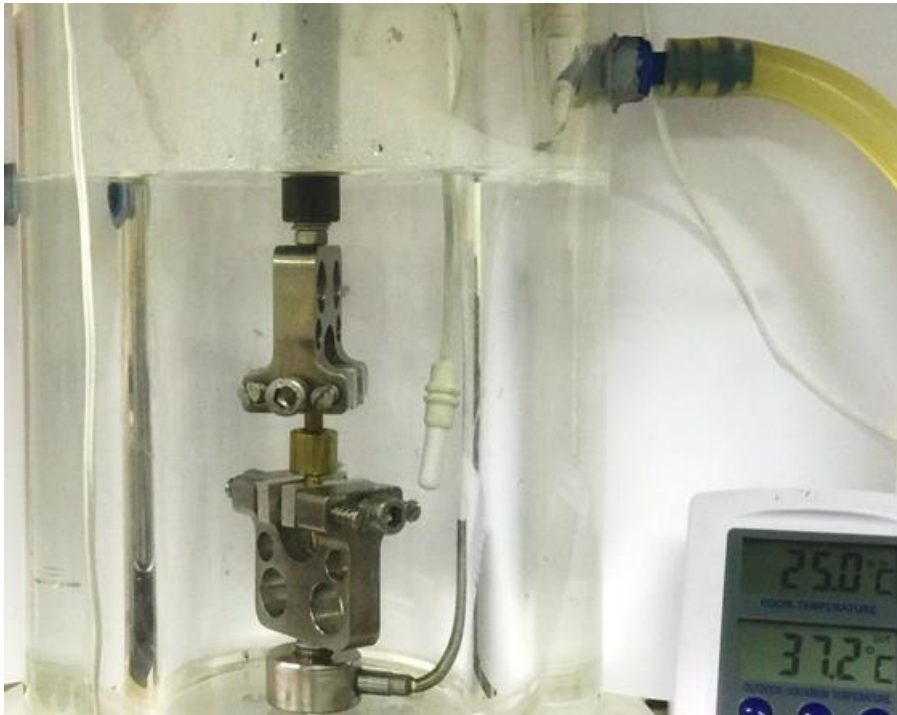
453 Figure 3: Testing of BDyn 1 device with degraded elastomer components in the custom built 454 chamber
