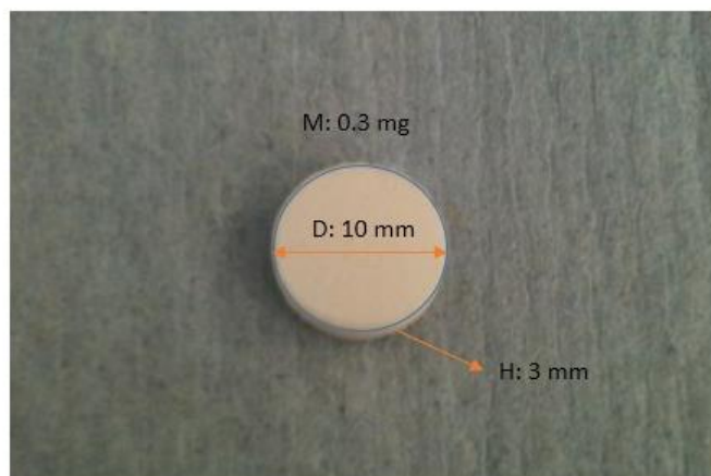
Fig.1 Graphic example of prepared tablet used for dissolution test
