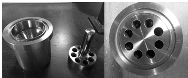
Fig. 1: Die design for open-ended tube extrusion.
