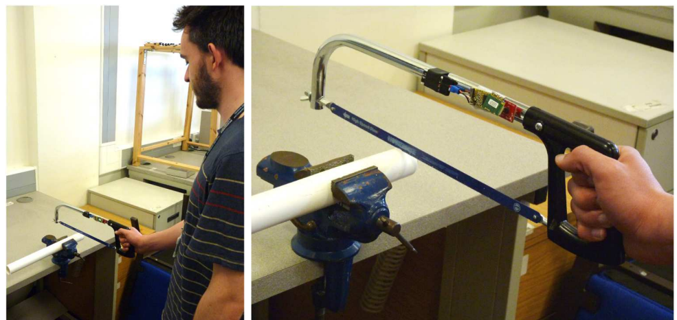
Fig 2. Data collection for experiment #4. Left: participant sawing into a plastic pipe, right: saw instrumented with accelerometer. The individual in this manuscript has given written informed consent (as outlined in PLOS consent form) to publish these case details.
