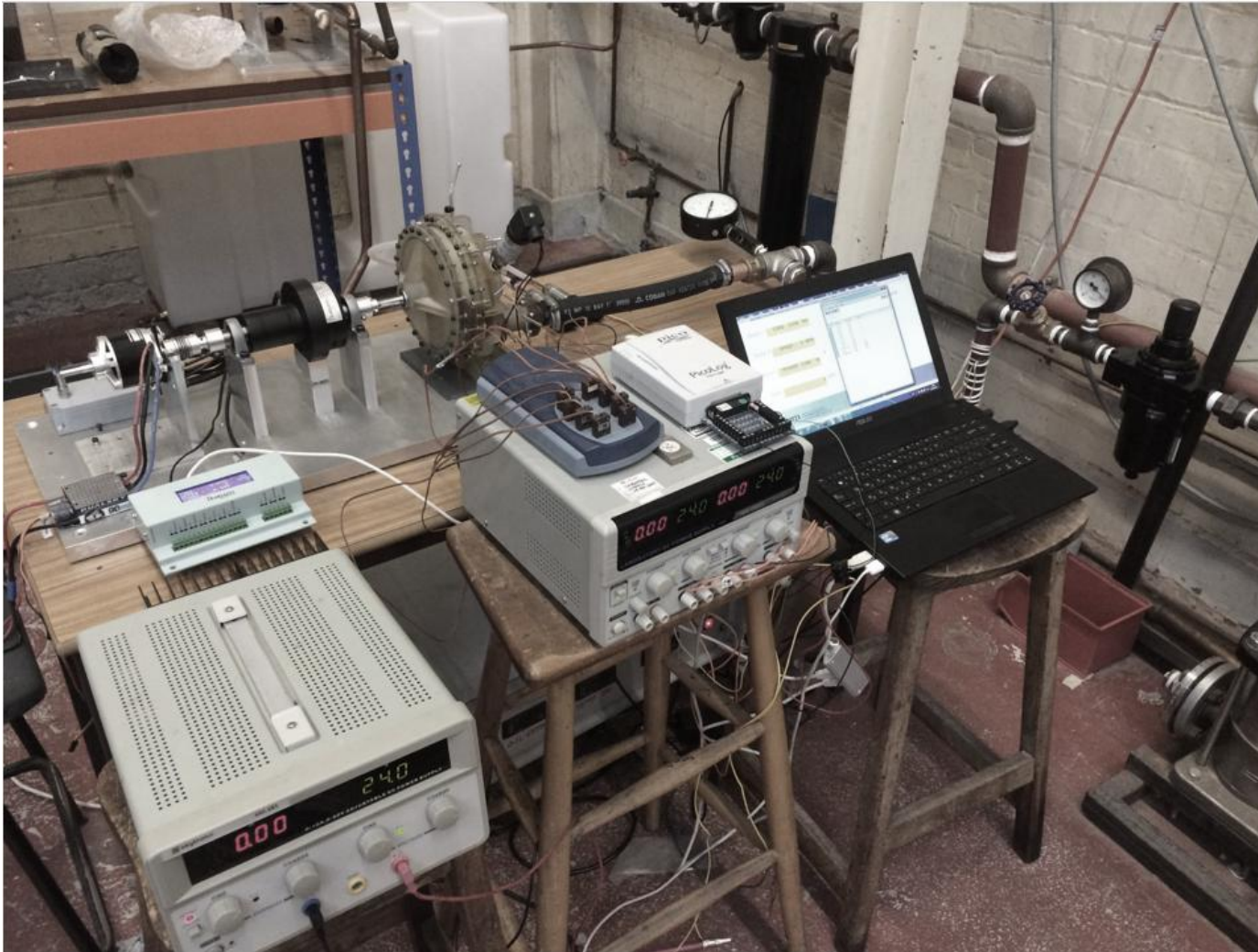
Figure 47 Fabricated experimental facility for testing the compressed air RIT
