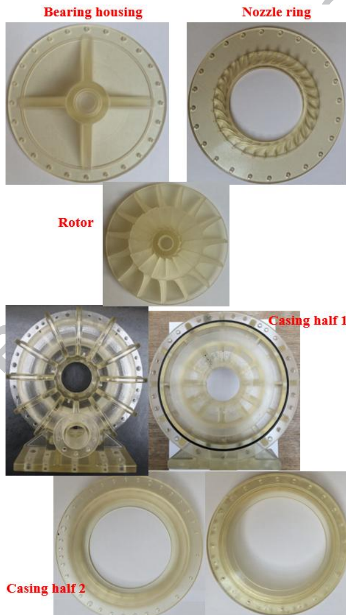
Figure 45 Manufactured turbine components with additive layer manufacturing technique
