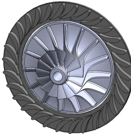
Figure 35 Final 3-D geometry of the rotor and nozzle
