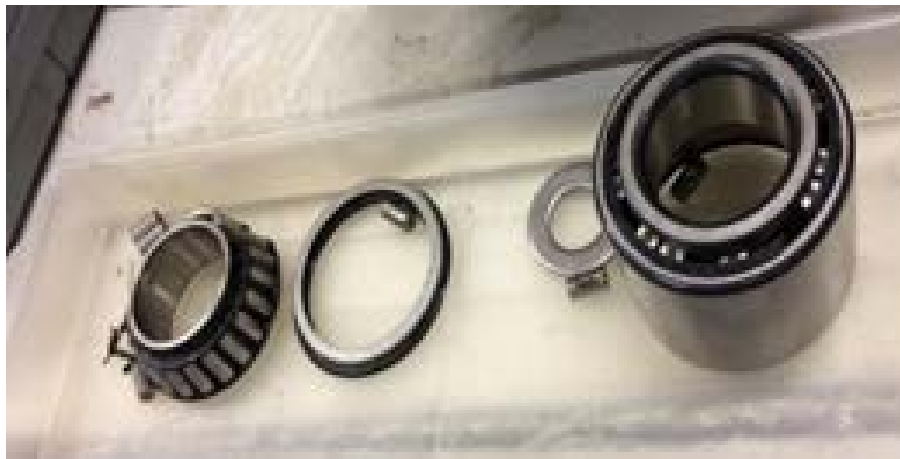
Figure 2: Example of a double-row tapered roller bearing using in the test rig laboratory experiments.
