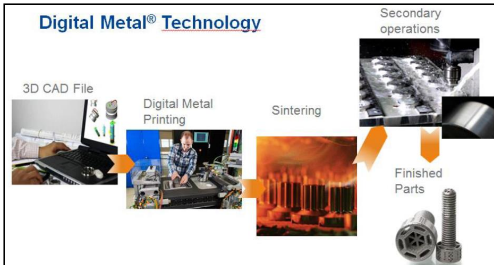
Fig. 2 Process diagram showing the Digital Metal® technology [43]
