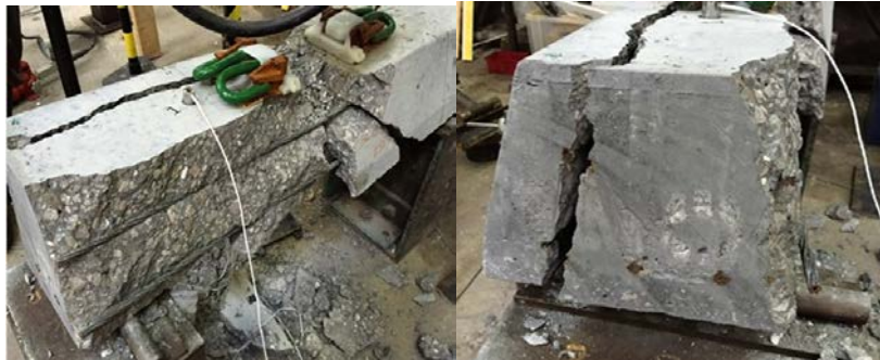
b) Sleeper with no web openings after loading
