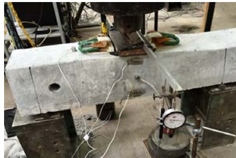
c) Sleeper with transverse hole before loading
