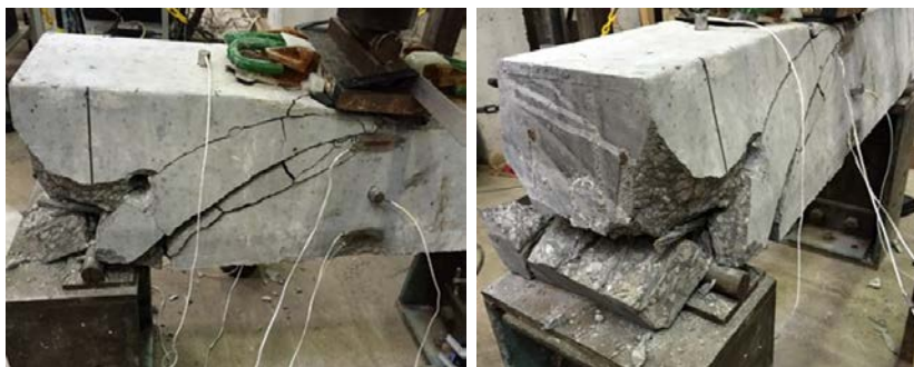
d) Sleeper with transverse hole after loading.
