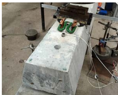
e) Sleeper with vertical hole before loading.
