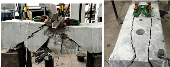
f) Sleeper with vertical hole after loading
