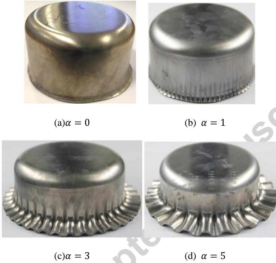
Fig. 3. Hot stamped parts using different blankholders
