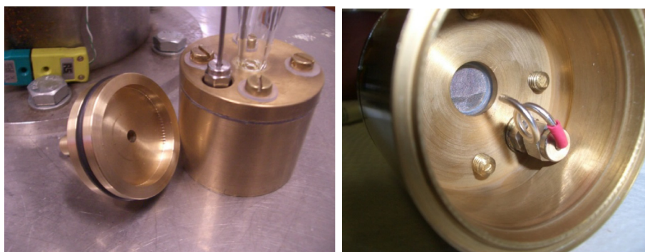
Fig. 2. Image of the plenum with the base of the glass fluidized bed attached, left; and underside of plenum showing nozzle tube to inject organic solution of API, right.
