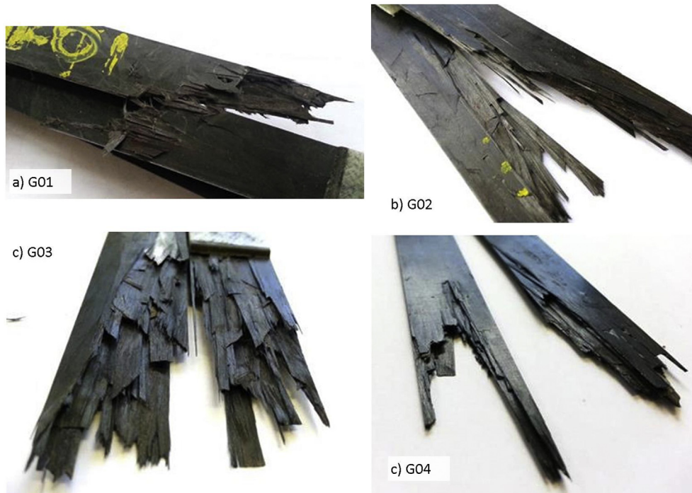
Fig. 10. Failure profiles of the tensile-tested coupons: a) G01, b) G02, c) G03 and d) G04.
