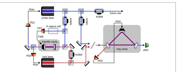
**Figure 2.** Simplified schematic of the cavity lock and probe laser systems. The lock laser operates at 852 nm and the probe laser at 770 nm. AOM: acousto-optic modulator; PD: photodiode; APD: avalanche photodiode; FMS: frequency modulation spectroscopy; PDH: Pound–Drever–Hall. All AOMs are in double-pass configuration. AOM1 tunes the probe beam, whose transmitted power is detected at the APD, AOM2 tunes the ring cavity, and AOM3/AOM4 are reserved for future experiments.
