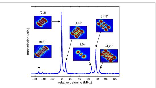
**Figure 3.** Transverse cavity modes. The solid curve shows a number of cavity transmission resonances (without atoms), and insets show the corresponding spatial profiles as imaged onto a camera. The  $45^{\circ}$  tilt of the patterns reflects the orientation of the cavity plane  $(\nwarrow_{\lambda})$ . The modes are labelled according to transverse indices (m, n), with asterisks denoting a longitudinal index q which is one less than that of the (0, 3) mode which is taken as reference.
