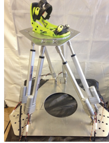
FIGURE 3: 6-DoF UPS parallel robot prototype built at the University of Birmingham.
