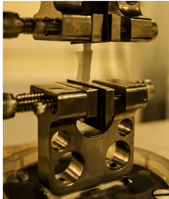
FIGURE 2. The specimen setup between the grippers, wrapped in tissue paper soaked in Ringer's solution and pre-loaded.
