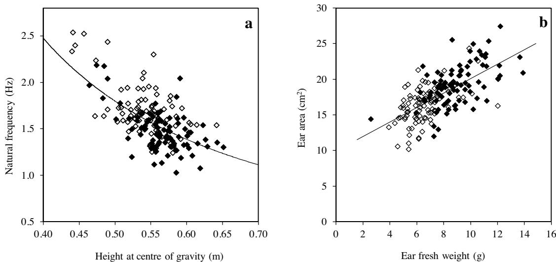
**Fig. 2.** (a) Height at centre of gravity at GS65+20 plotted against natural frequency for plot means of 2012 (closed squares) and 2013 (open squares). Regression line:  $y = 0.67x^{-1.4}$  ( $R^2 = 0.38$ ;  $P < 0.001$ ). (b) Ear fresh weight plotted against ear area at GS65+20, for plot means of 2012 (closed squares) and 2013 (open squares). Best fit line:  $y = 1.02x + 9.95$  ( $R^2 = 0.44$ ;  $P < 0.001$ ).
