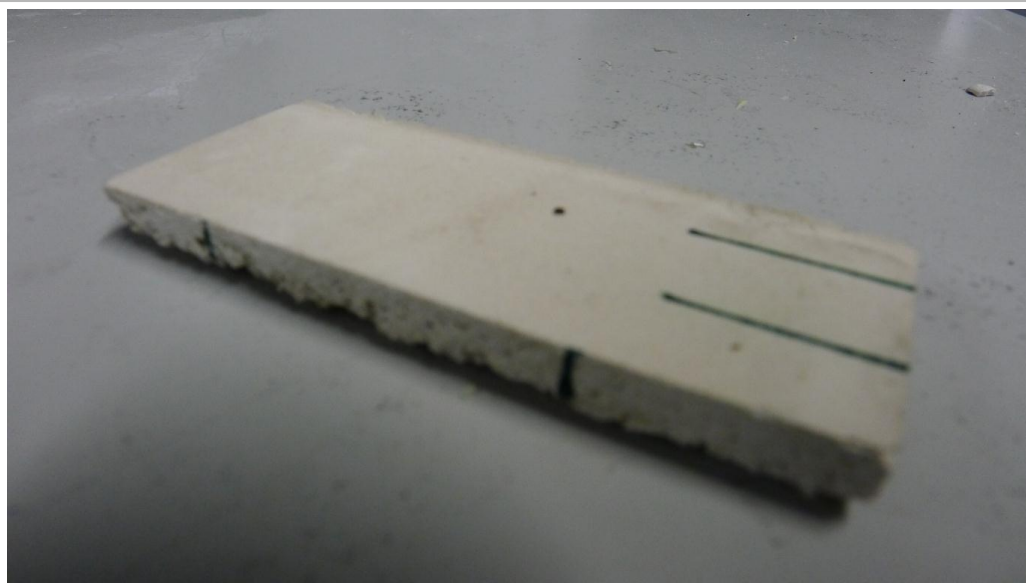
Figure 4- The width and thickness of each sample is noted with line to assure the same location is being measured.
