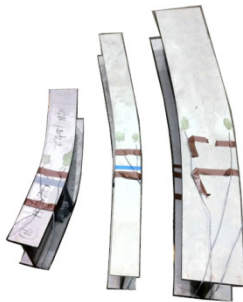
Fig. 13. Typical failure modes for minor flexural buckling.
