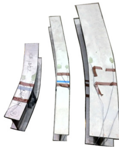
Fig. 13. Typical failure modes for minor flexural buckling.
