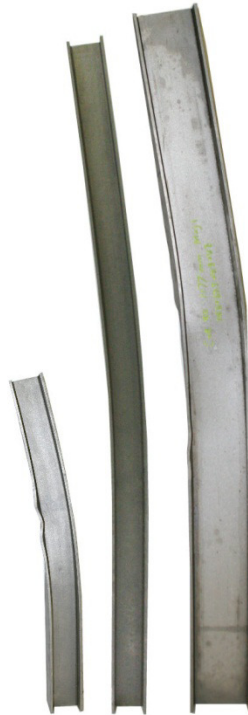
Fig. 16. Major flexural buckling failure modes.
