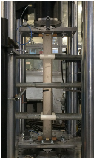
Fig. 15. Major flexural buckling test setup.
