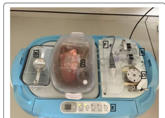
Fig. 1 LifePort Kidney Transporter 1.0 (Organ Recovery Systems) containing a porcine kidney. a Bubble chamber. b Reservoir for ice. c Aortic patch connector for perfusion. d Peristaltic pump. e Controls (pressure, prime, wash, infuse). f Sampling port
