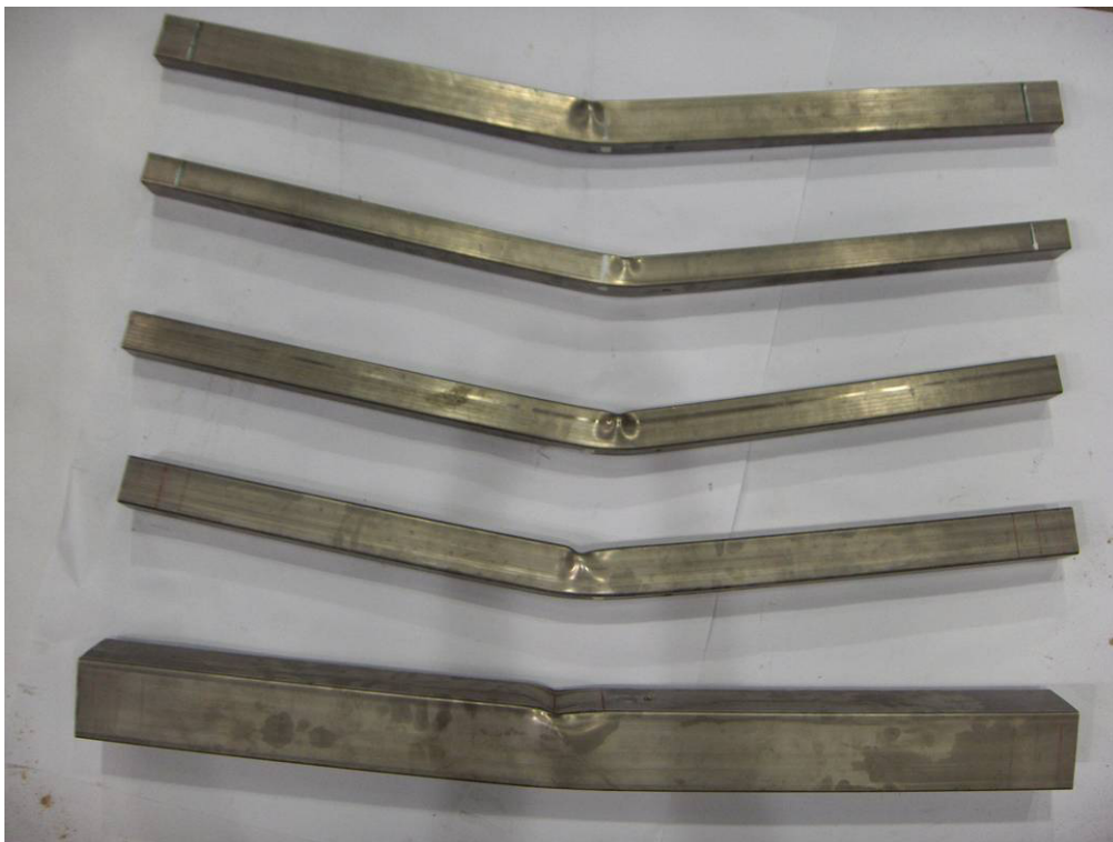
Fig. 4. Failure modes for simply supported RHS and SHS beams (from top to bottom RHS 60x40x3-MA, RHS 60x40x3-MI, SHS 50x50x3, SHS 60x60x3, SHS 100x100x3).
