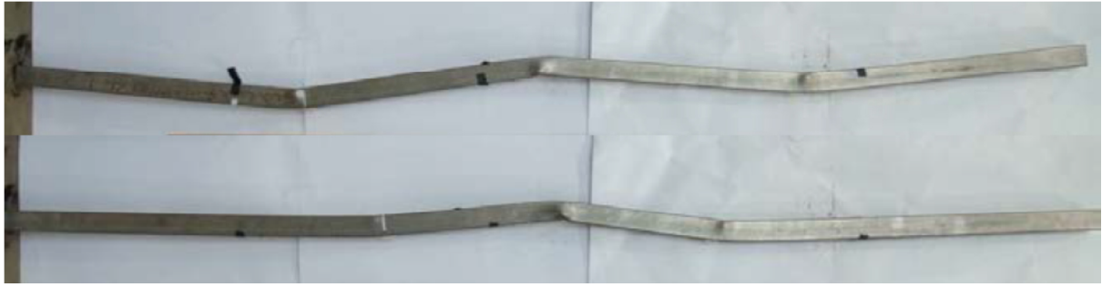
Fig. 14. Failure modes of SHS 50×50×3-1 – configuration: 1/2 span (top) and SHS 50×50×3-2 – configuration: 1/3 span (bottom).
