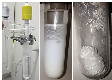
Fig. 2 Images of a typical [\text{NH}_4][\text{OTf}] -catalysed silicon imidonitride preparation immediately after warming to ambient temperature (left, showing the side-arm used to measure liquid ammonia), after gelation at 24 h aging time (centre), and the xerogel after solvent removal (right).
