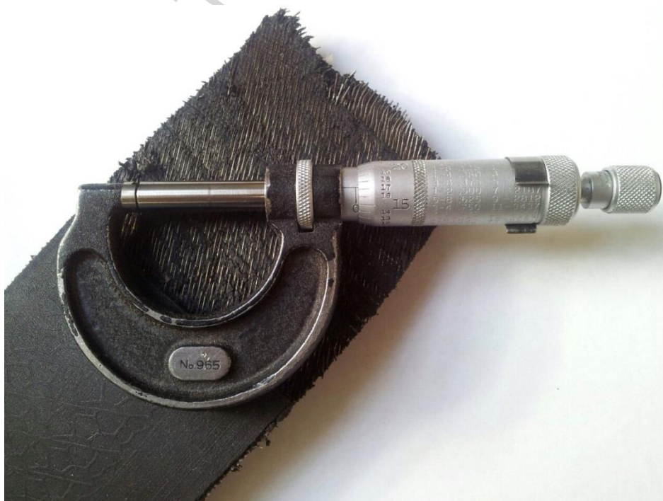
Figure 3 Measurement for cross-section area of steel cord
