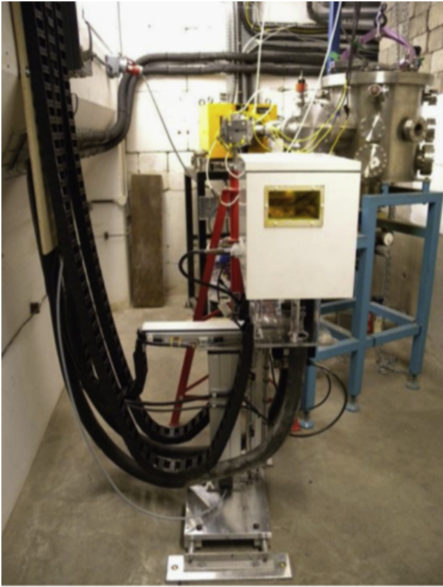
Fig. 1. The scanning system and cold box in the Birmingham Irradiation Facility.
