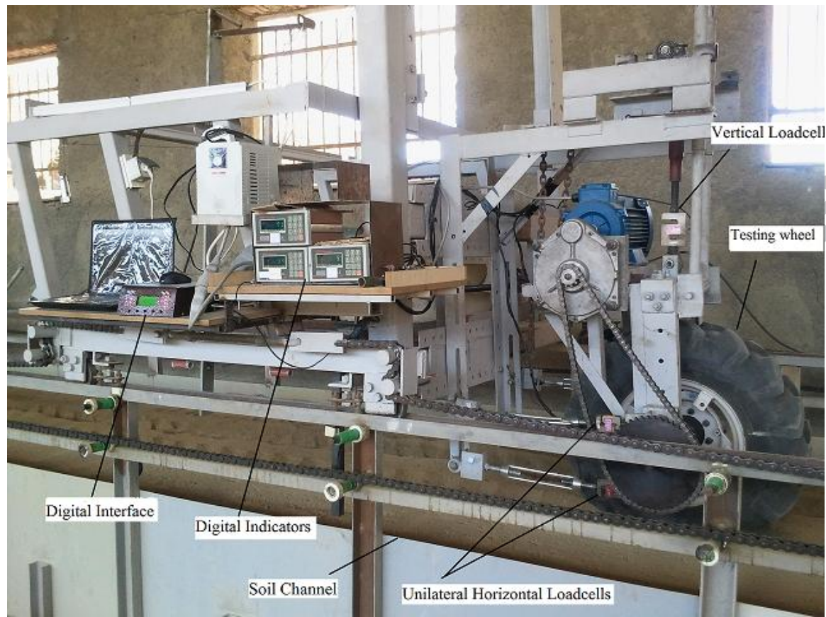
Figure 2- Soil bin testing facility and the components
