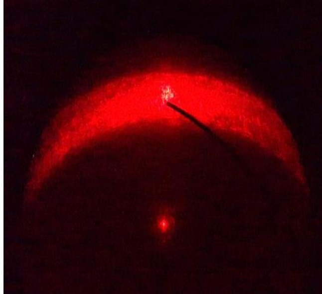
Fig 7. An example of a diffraction pattern from a spherulite produced on the semi-transparent hemispherical screen in Fig. 1.
