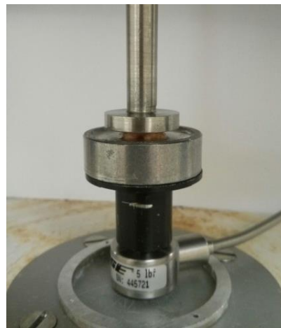
Figure 2 – Compressive DMA set-up for human bladder tumours.
