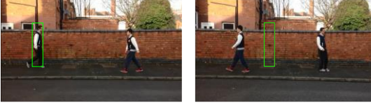
Figure 3. Failure modes in environmental clutter. In this case, the target walks from left to right across the scene, but is temporarily occluded by a distracting object, sharing similar feature values, which passes from right to left.
