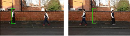
Figure 3. Failure modes in environmental clutter. In this case, the target walks from left to right across the scene, but is temporarily occluded by a distracting object, sharing similar feature values, which passes from right to left.
