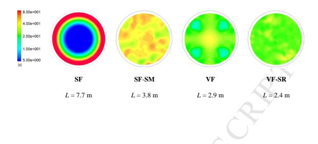
Figure 13. Radial contour plot of C-value at the exit section of heating tubes with different flow regimes achieving the same mean sterility ( $\overline{F} = 37.6$  s) at the exit section (note that the red colour in the **SF** plot is ~ 4-fold greater than the top end of the scale).
