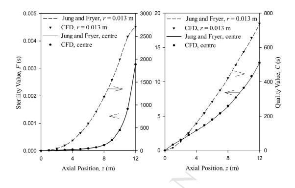
Figure 4. Validation of CFD-predicted axial profiles of sterility and quality of an isoviscous fluid in steady-state flow in a heating tube against simulation results from Jung & Fryer (1999), for the processing conditions of Table 3.
