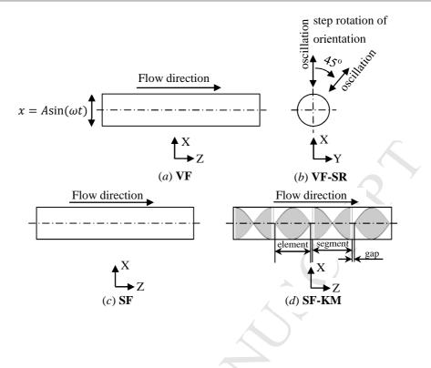
Figure 1. Flow configurations: (*a*) flow through a tube subjected to transverse oscillations (**VF**); (*b*) flow through a tube subjected to transverse oscillations with step rotation of vibration orientation (**VF-SR**); (*c*) steady flow through a tube (**SF**); (*d*) steady flow through a tube fitted with a Kenics static mixer (**SF-KM**), showing 4 elements out of 48.
