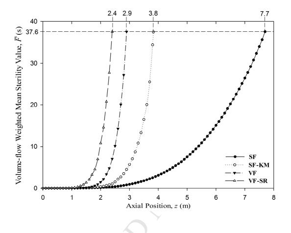
Figure 12. Axial profile of mean F-value in heating tubes with different flow regimes achieving the same mean sterility ( $\overline{F} = 37.6$  s) at the exit section.
