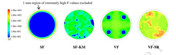
Figure 8. Radial contour plot of F-value at the exit section of the heating tube.
