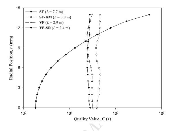
Figure 14. Radial profile of azimuthally-averaged C-value at the exit section of heating tubes with different flow regimes achieving the same mean sterility ( $\overline{F} = 37.6$  s) at the exit section.
