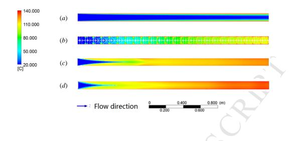
Figure 7. Axial contour plot of azimuthally-averaged temperature in the heating tube: (*a*) **SF**; (*b*) **SF-KM**; (*c*) **VF**; (*d*) **VF-SR**.
