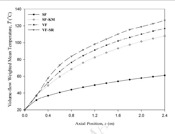
Figure 6. Axial profile of mean temperature in the heating tube.
