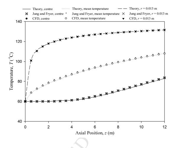
Figure 3. Validation of CFD-predicted temperature profiles of an isoviscous fluid in steady-state flow in a heating tube against theory (Jakob, 1949) and simulation results from Jung & Fryer (1999), for the processing conditions of Table 3.
