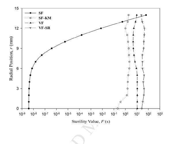
Figure 9. Radial profile of azimuthally-averaged F-value at the exit section of the heating tube.
