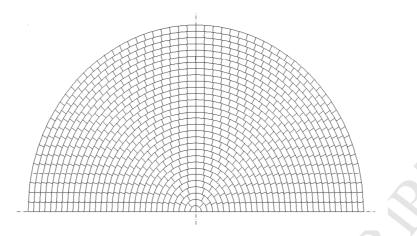
Figure 2. Illustration of grid used on MATLAB for evaluation of volume-flowrate weighted mean temperature, sterility and quality over tube cross-section (total number of cells, N = 1860 cells).
