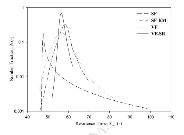
Figure 10. Fluid residence time distribution in the heating tube.
