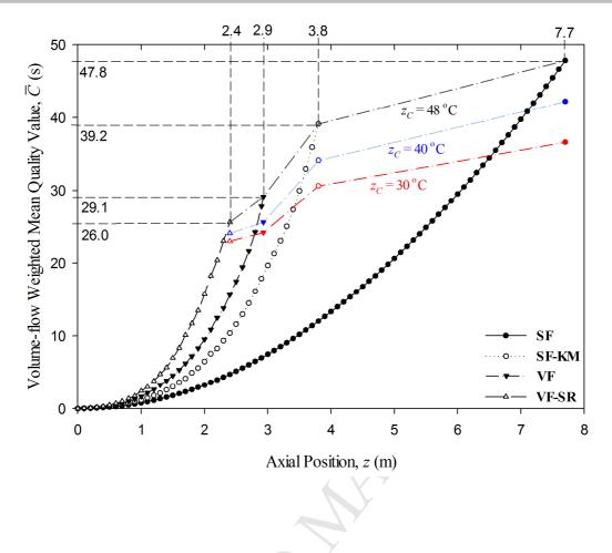
Figure 15. Axial profile of mean C-value in heating tubes with different flow regimes achieving the same mean sterility ( $\overline{F} = 37.6$  s) at the exit section.
