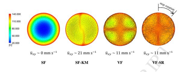
Figure 5. Radial temperature and velocity vector distributions at the exit section of the heating tube.
