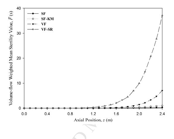
Figure 11. Axial profile of mean F-value in the heating tube.
