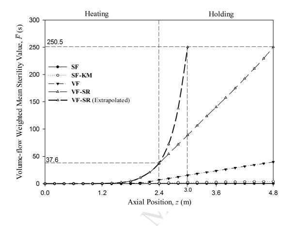
Figure 16. Development of mean F-value along heating and holding tubes.
