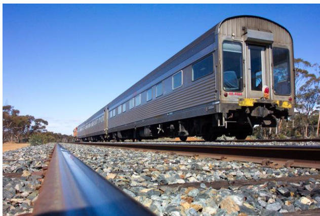
Fig. 3 AK Car, a track inspection train
