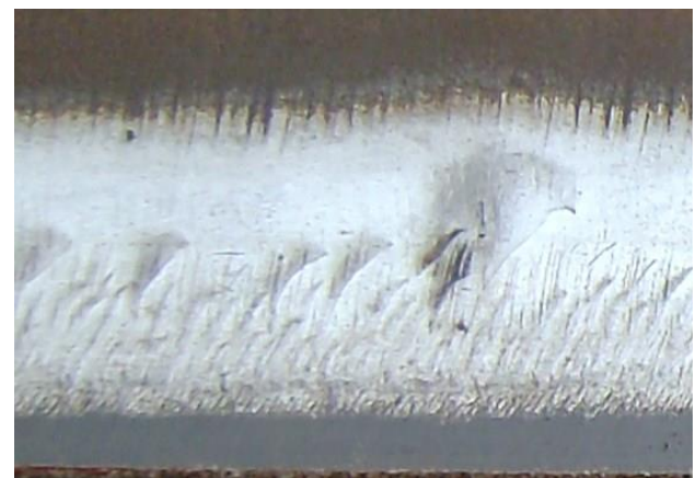
b) Close up for visible Cracks Fig. 5 Rail squats in the field
