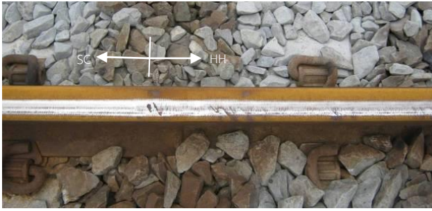
Fig. 7. Interface between SC rail and HH rail. The SC rail is squat free. Squats are visible at the weld and in the HH rail. High rail in transition to 932m radius curve [5].
