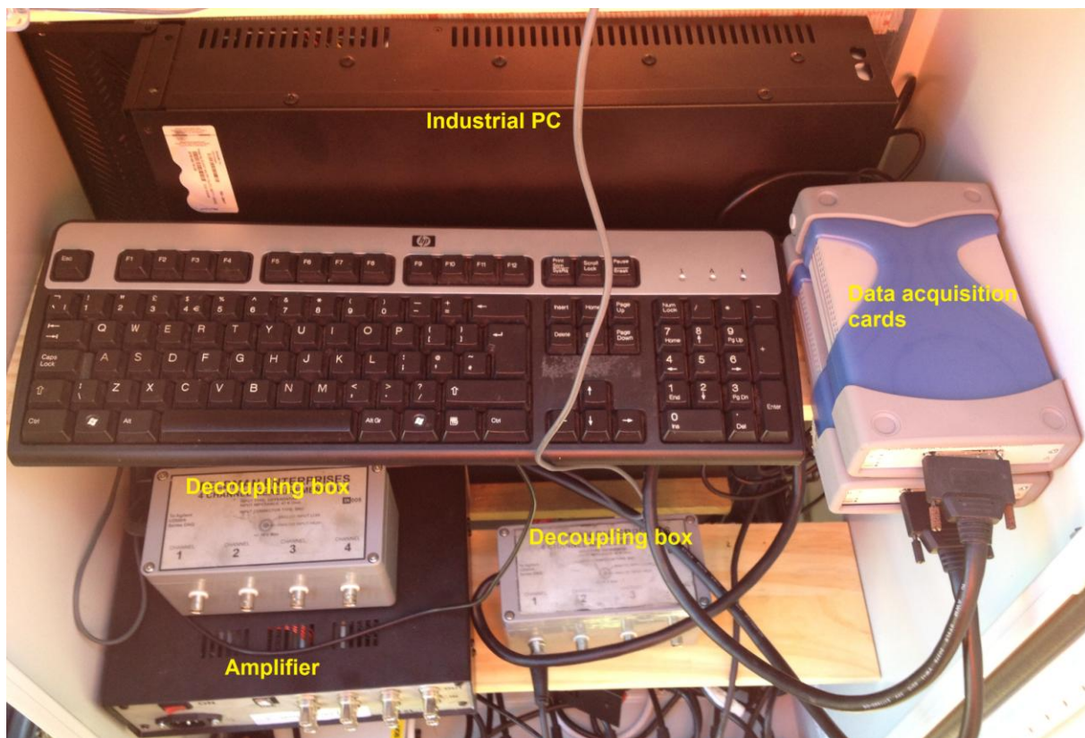
Figure 7: The customised data acquisition equipment used during trials in Long Marston.
