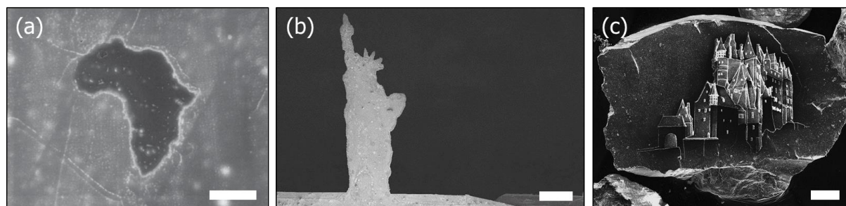
Figure 4. Microfabricated artwork by focused ion beam milling (FIBM). (a) Actual Size. Scale bar = 100 nm. Reproduced with permission. [70b] Copyright, 2007 Macmillan Publishers Ltd. (b) Probation. Courtesy of Alessandro Scali and Robin Goode, 2007. Scale bar = 100 \mu\text{m} (c) Sandcastle draft of Eltz Castle (Germany) on a sandgrain. Single pixel resolution = 50 nm, single line = 0.4-1.0 \mu\text{m} , scale bar = 50 \mu\text{m} . Courtesy of Marcelo Coelho and Vik Muniz.
