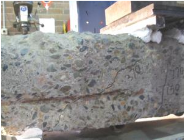
Figure 16 Damage on the sleepers (a) a flexural crack and a diagonal crack on the sleeper UOW7, (b) a wide flexural crack on the sleeper UOW8.
