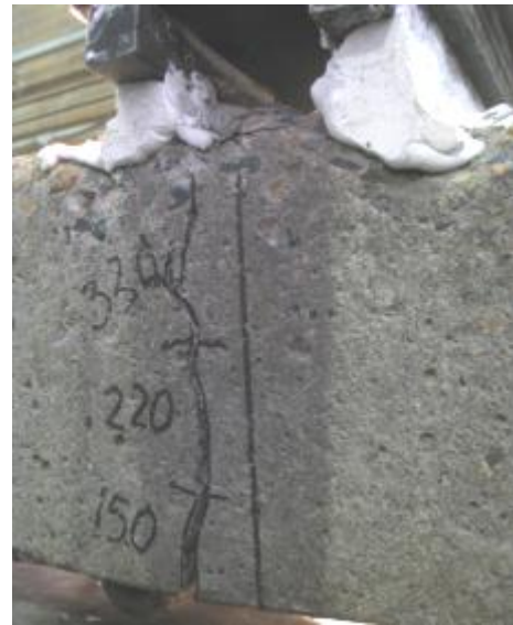
Figure 16 Damage on the sleepers (a) a flexural crack and a diagonal crack on the sleeper UOW7, (b) a wide flexural crack on the sleeper UOW8.
