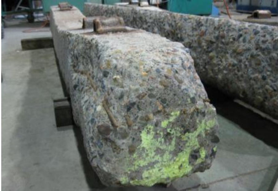
g) damage of concrete at the end and one prestressing wire was exposed in sleeper UOW7
