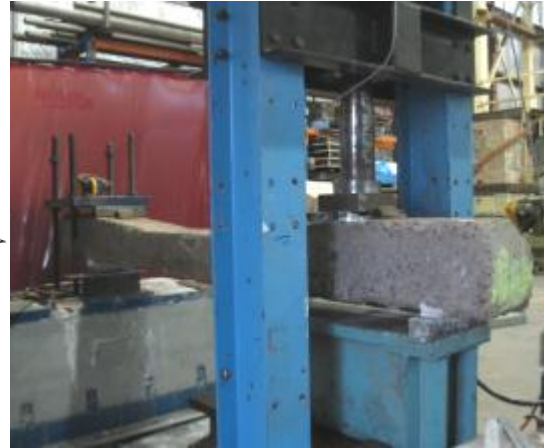
Figure 5 (a) and (b) - Rail seat vertical load static test for negative bending moment
