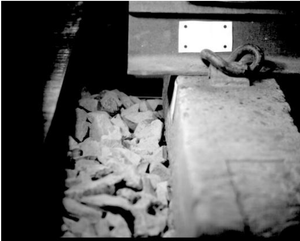
Figure 35 High-speed recording of sleeper response in soft track condition
