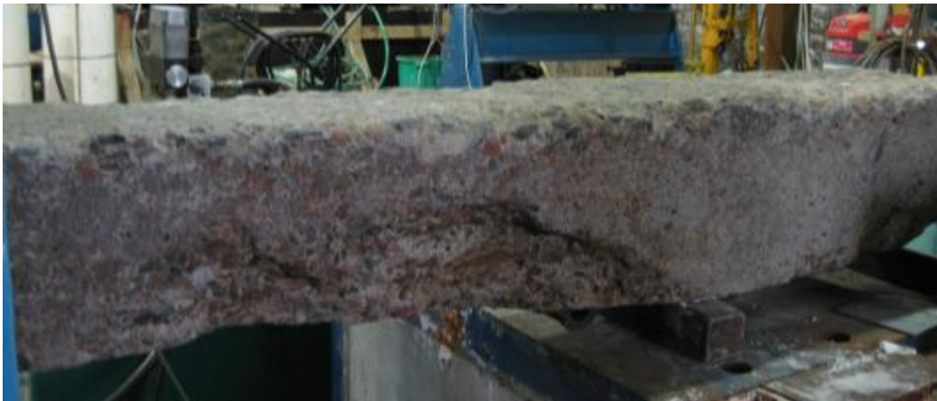
726 727 d) severe damage of concrete between the mid-span and the support for the sleeper UOW4
