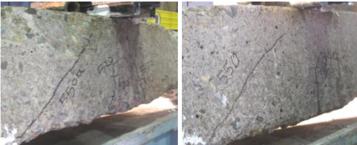
Figure 13 Damage of sleepers under rail seat positive moment test (a) flexural cracks and diagonal crack for sleeper UOW5 and (b) flexural crack and diagonal crack for sleeper UOW6.
