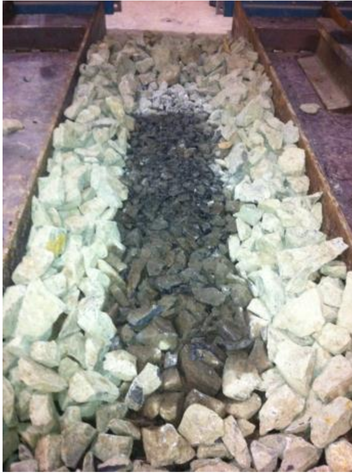
Figure 28 Crushing of ballast underneath concrete sleeper due to impact loads
