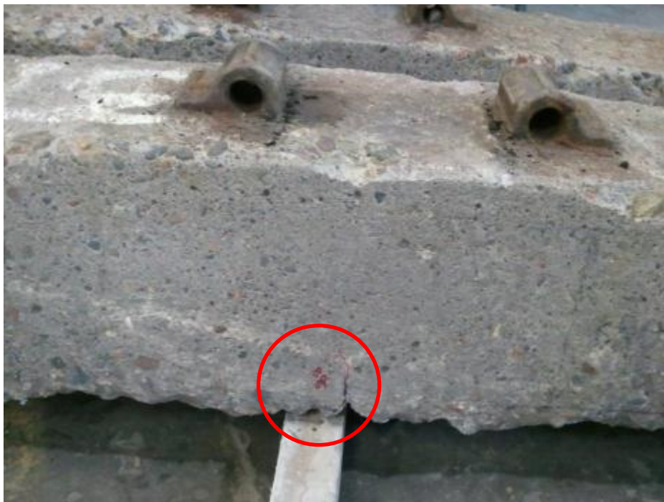
Figure 27 Minor cracking at rail seat starting from soffit surface
