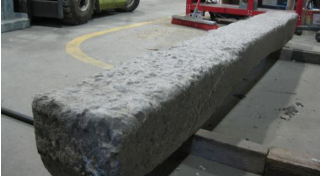
a) severe abrasion of concrete cover at the bottom surface of the sleeper UOW1
