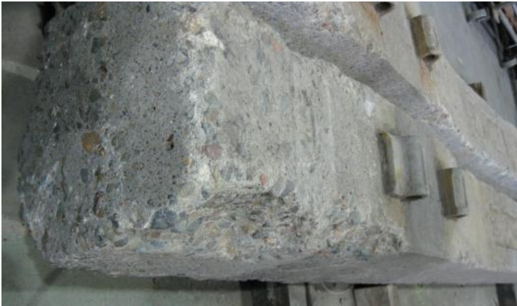
b) concrete damage at the end of the sleeper UOW2
