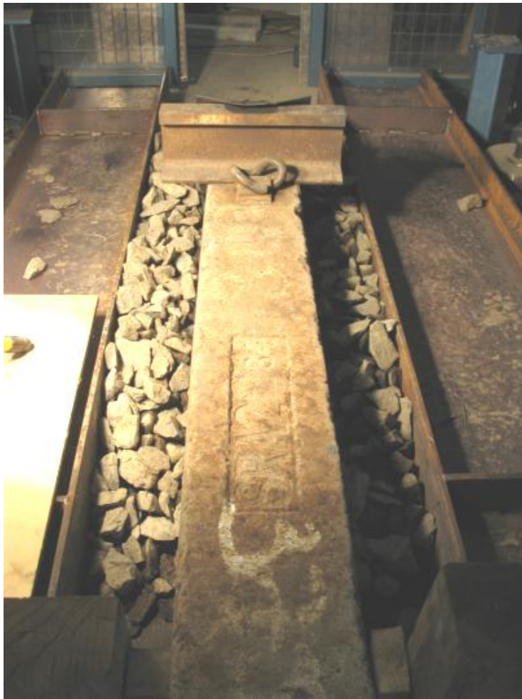
Figure 22 Experimental modelling of hard track support condition
