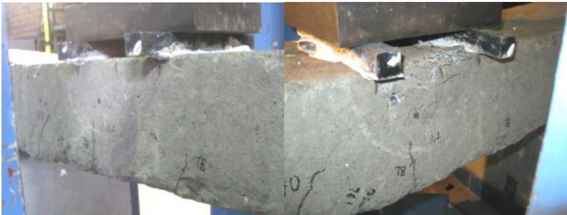
Figure 19 (a) Cracking of sleeper at mid-span for UOW1, and (b) crushing of concrete at the top for UOW1.
