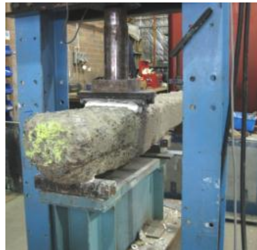
Figure 6 (a) and (b) - Rail seat vertical load static test for positive bending moment
