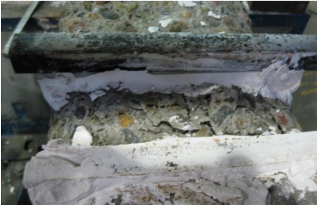
Figure 17 Crushing of concrete in compression for the sleeper UOW8.
