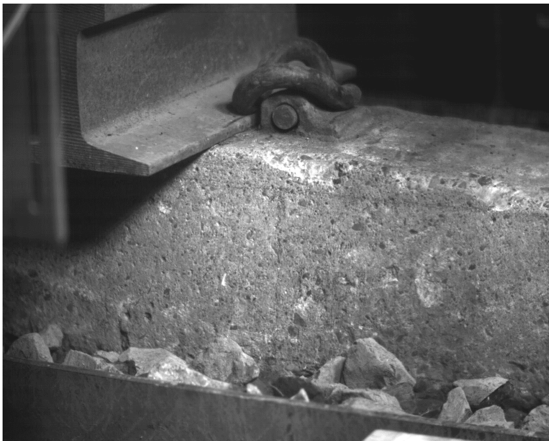
Figure 25 High speed recording of dynamic response of sleeper in hard track condition
