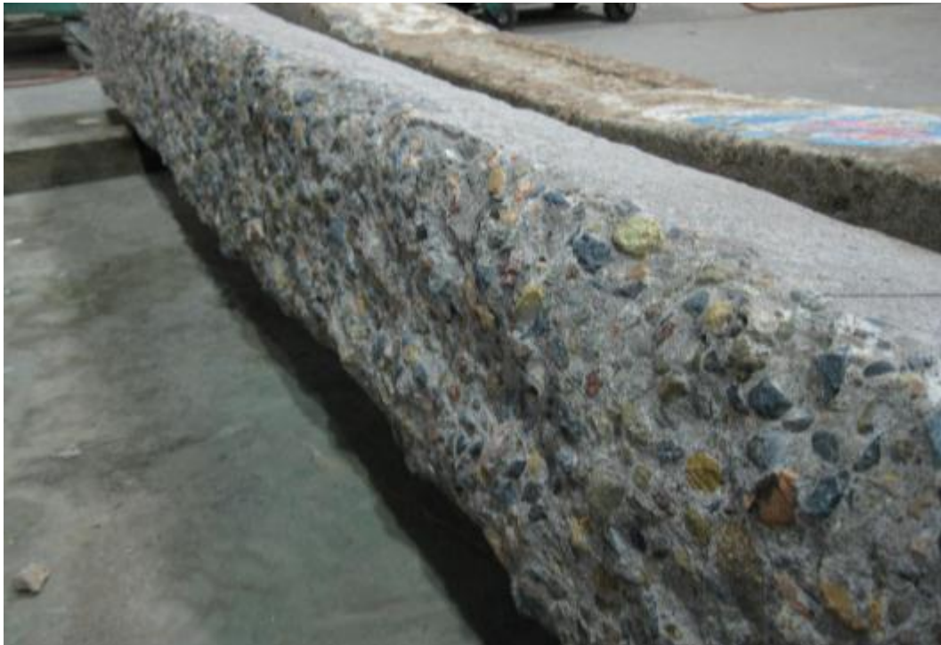
h) very severe abrasion on the concrete cover at the bottom surface of sleeper UOW8
