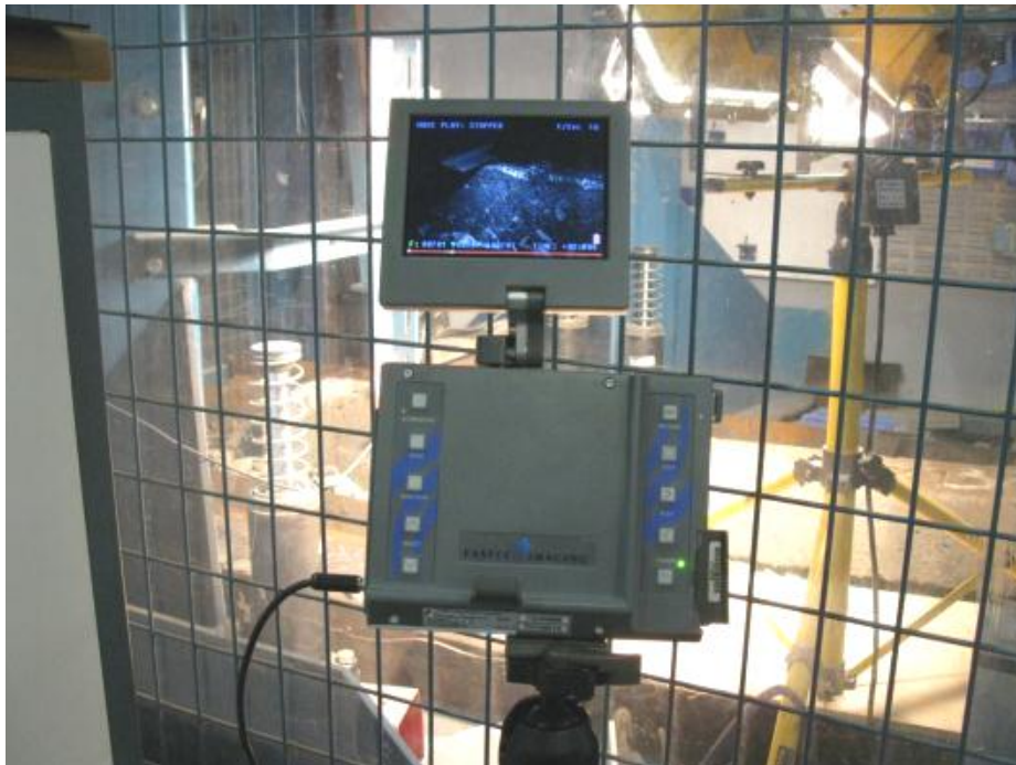
Figure 23 High speed camera for recording dynamic response of concrete sleeper
