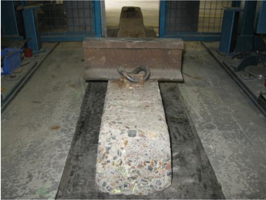
Figure 29 Experimental modelling of medium track support condition
