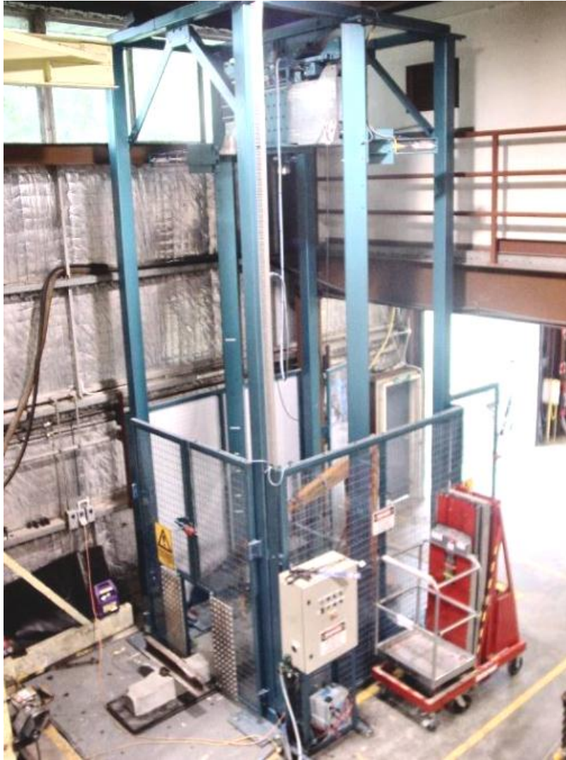
Figure 9 Drop hammer facility at UoW
