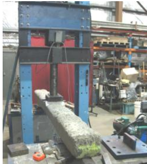
Figure 7 (a) and (b) - Sleeper centre vertical load test for negative bending moment
