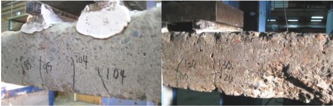
Figure 21 (a) Cracking of sleeper at mid-span for UOW3, and (b) Cracking of sleeper at mid-span for UOW4.
