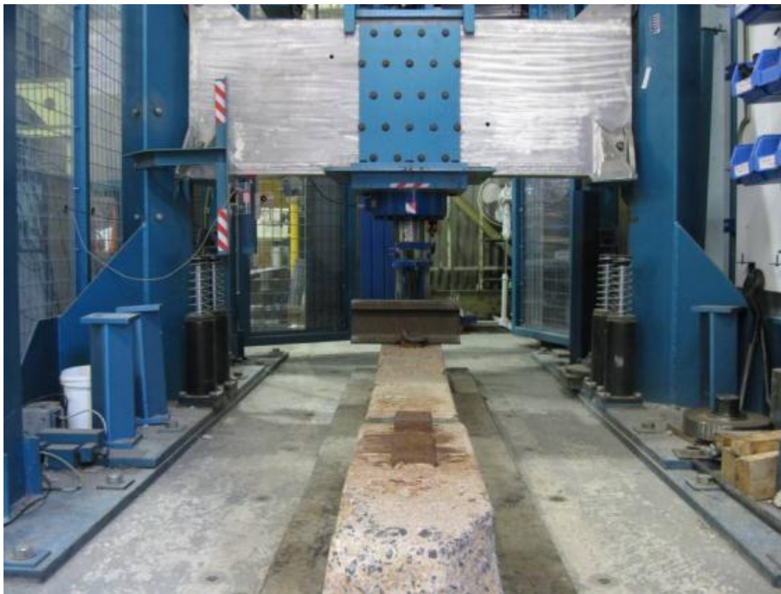
Figure 11 Impact testing of coal-line concrete sleepers at rail seat
