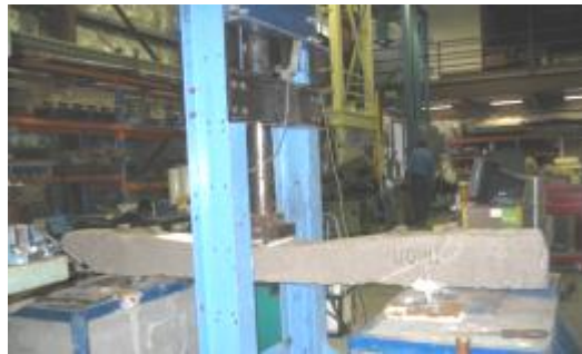
Figure 8 (a) and (b) - Sleeper centre vertical load test for positive bending moment
