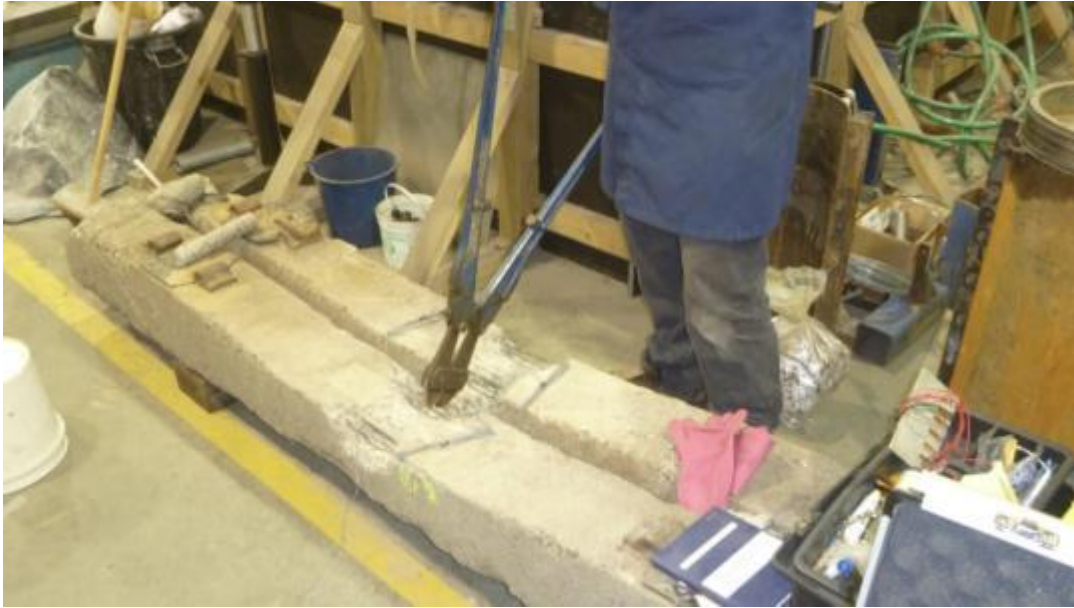
Figure 7. Cutting of prestressing wires
