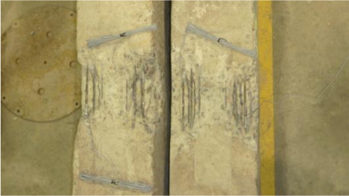
Figure 5. Preparation of specimens for dynamic relaxation tests
