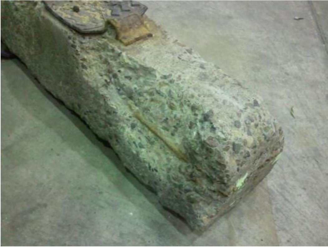
Figure 10. Sleeper end damage possibly resulting in considerable loss of prestress
