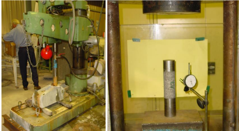
Figure 3. Preparation of concrete samples (left: coring machine; and right: cored concrete samples prior to compression testing).
