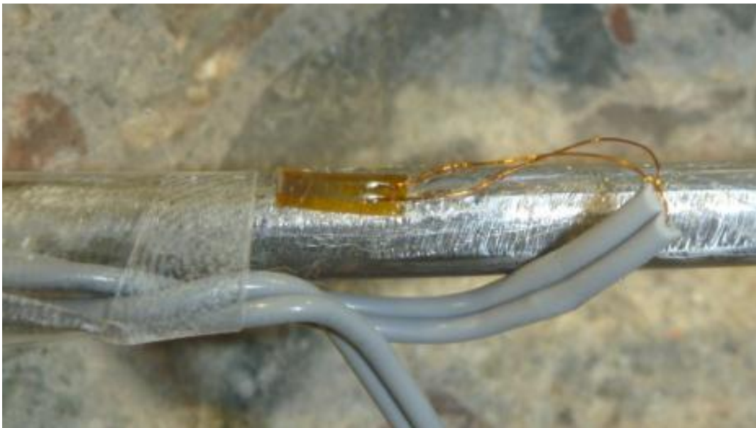
Figure 6. Two-millimetre strain gauges attached to prestressing wire
