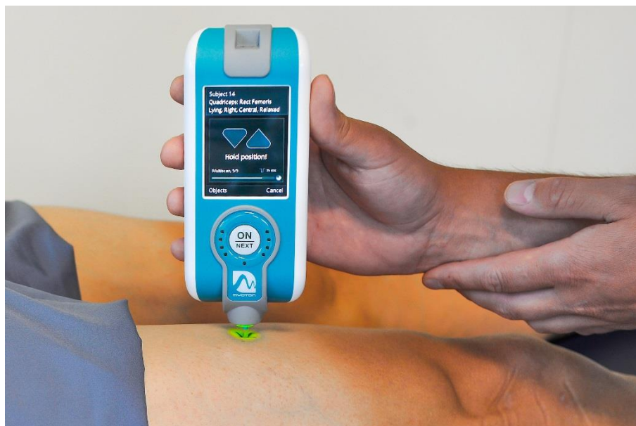
Figure 2. MyotonPRO technique for measurement of rectus femoris (RF) stiffness, tone and elasticity
