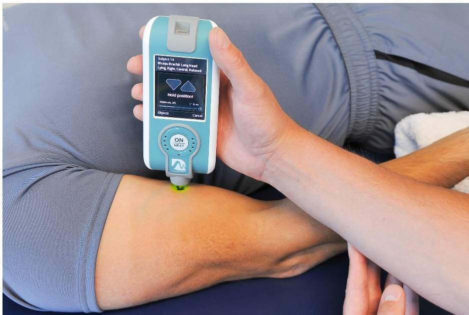
Figure 1. MyotonPRO technique for measurement of biceps brachii (BB) stiffness, tone and elasticity
