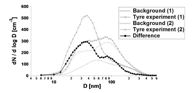
**Figure 3.** SMPS size distributions of the tyre experiment (and relative background). The difference (average of diff exp 1 and diff exp 2) shows an enhancement of particles at 35 and 85 nm.
