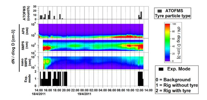
**Figure 2.** The tyre dust lab experiment. Top chart shows the Art-2a ATOFMS particle type associated to tyre dust (ATOFMS counts/hour), middle charts show aerosol size distributions (APS, SMPS, nano-SMPS) and bottom chart shows the experimental mode used.
