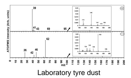
**Figure 4.** ATOFMS art2a cluster associated with tyre dust in the laboratory.
