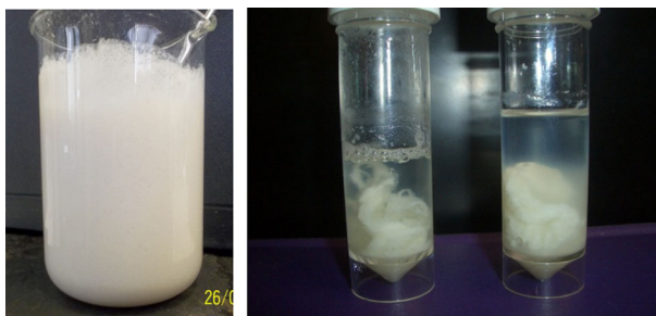
Fig. 4 Images of bactofuge desludge pre- (left) and post- (right) EPS treatment. Process conditions: batch; 100 bar CO 2 , 300 W pulsed sonication power, 3 min
