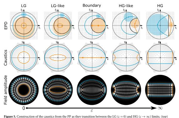
Figure 5. Construction of the caustics from the PP as they transition between the LG (c = 0) and HG ( $c \to \infty$ ) limits. (top) Equatorial Poincaré disk (EPD) with the projection of the PP (inner black curve) and the two medial axes (blue and orange curves) with examples of the bitangent circles used to construct them, (middle) the caustics obtained via the conformal mapping of the medial axes and (bottom) the caustics overlaid on top of amplitude distribution of the corresponding beam.
