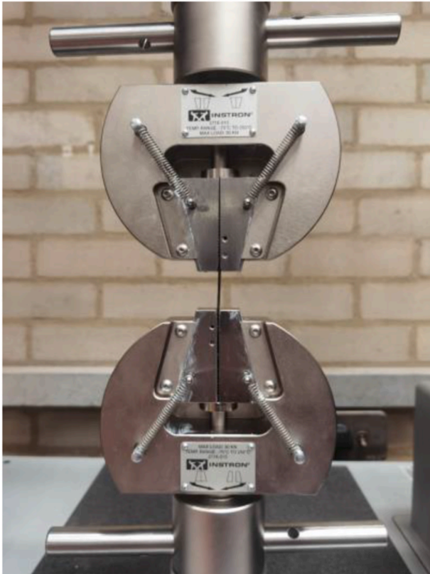
Fig. 2. Test setup for tensile strength test of RSF.
