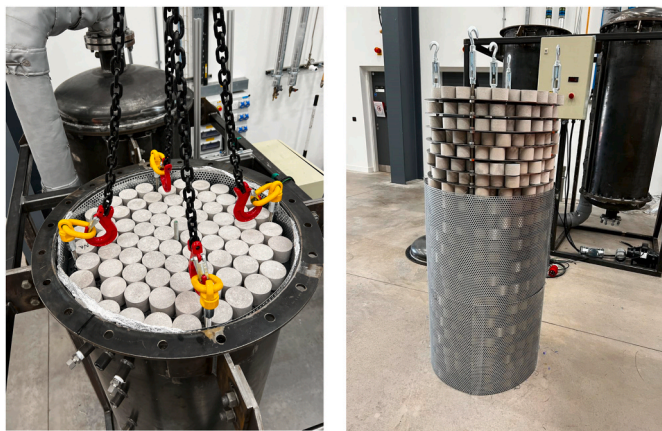
Fig. 3. Left: Tank trays with pellets loaded in the tank using a lift crane. Right: Stack of pellet covered trays half covered with aluminium foil.
