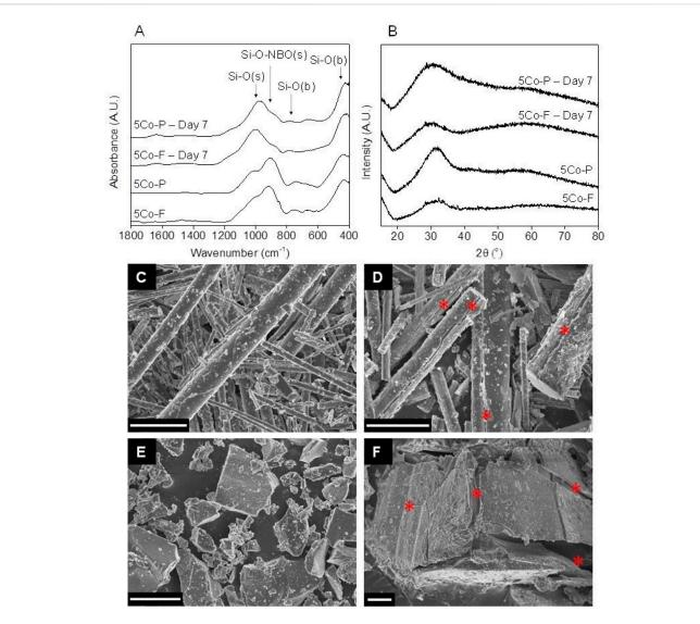
FTIR (A) and XRD (B) of the glasses containing cobalt before and after incubation in DMEM for 7 days: 5Co fibres (5Co-F) and particles (5Co-P); SEM images of 5Co-F before (C) and after (D) incubation in DMEM for 7 days, and 5Co-P before (E) and after (F) incubation in DMEM at a concentration of 1.5 mg ml<sup>-1</sup>. Scale bar is 10  $\mu$ m, and \* indicates cracks forming in the fibres and particles after incubation in DMEM.
