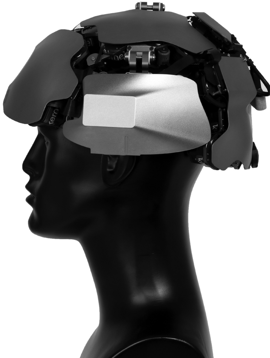
Fig. 1 Side view of the modules and structural plates that make up the Flow system. Each plate of modules establishes a fixed distance between the sources and detectors of the modules within the plate. The spacing between plates can be controlled using spacers that should be adjusted based on the user's head size and desired regions of interest.
