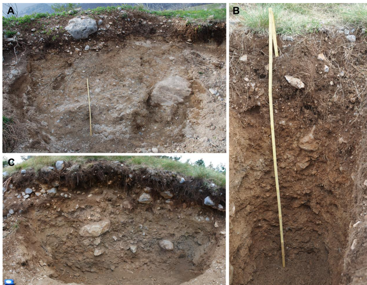
Fig. 3. Cleared sections of three studied tills: A) homogenous, massive, matrix supported till unit of Jovići Moraine; the scale is 1 m in length. The upper 0.5 m of the section are sediments mobilized decades ago when the pit was originally excavated. B) Massive, clast supported, homogeneous till of Rujnička Kosa moraine. The scale is 1.8 m in length. C) Internal Trench moraine till with two identified units, see figure 5 for stratigraphy details. The trench is 2 m in height.
