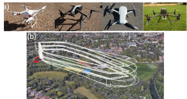
FIGURE 6 (a) Left-to-right DJI Phantom 3 (P3-D), DJI Inspire 2 (I3-D), DJI Mini Mavic 2 (M2-D), and DJI Matrice 300 (MT-D) drones. (b) Google Earth plot of GPS tracks from a control trial.
