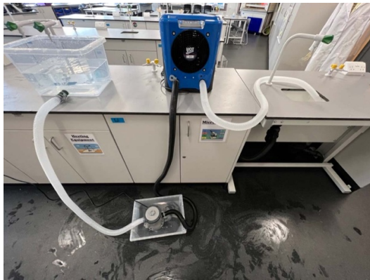
Figure 3. Photograph of the air source heat pump experimental setup.
