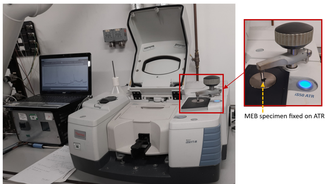
Figure 2. Experimental setup (FTIR-ATR) and a zoom-in of the specimen fixed on the ATR.
